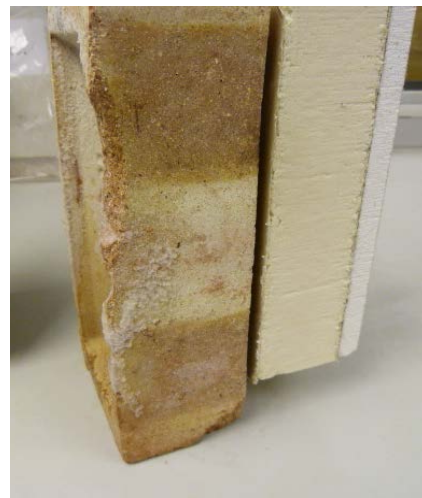
Photos 1 & 2: Left hand side shows the appearance during the test and the right afterwards with crystallising salts
