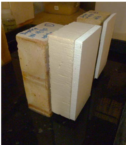
Photos 1 & 2: Left hand side shows the appearance during the test and the right afterwards with crystallising salts
